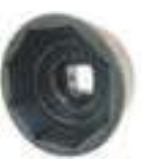
H.C.B-A1404 ROR TRAILER REAR WHEEL NUT SOCKET (Dr. 1", 8 POINT, 83 mm, 3 1/4") (DRUM BRAKE) ROR 板車輪軸螺帽套筒 (Dr. 1", 8 角, 83 mm, 3 1/4") (鼓式煞車)
